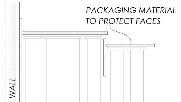
4. Screw leg bases to bottom of lower cases. Lines on the bottom of the case indicates set back from both front and back. Standard inset on gabled sides is with the leg base tab supporting the gable end.
